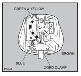
The wire coloured green and yellow must be connected to the terminal marked with the letter «E» or by the earth symbol  $\frac{1}{2}$  or coloured green and yellow.
